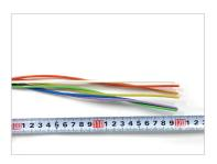
4. Prepare a cable. Measure 120cm and remove cable sheath.
