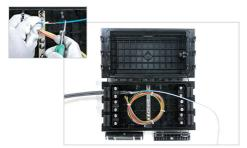
9. Separate the loose tube cable unit to splice and arrange the rest. Remove buffer tube of the loose tube cable unit to splice, leaving 10cm. Remove jelly on the fibers. Insert the protection tube to the fibers and protect the fibers.
