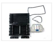
1. Prepare the closure. Remove Velcro strap and uninstall the splice trays. Remove gasket from the gasket track.
