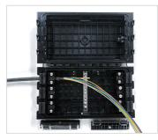
8. Retain the cable with the cable clamp. **Attention!** Do not tighten the cable clamp too much as it causes optical loss.
