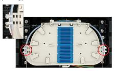
11. Install the splice trays. Bring the fibers to the splice tray and retain them to the splice tray with cable ties.
