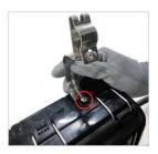
14. Attach the mounting brackets to the closure.
