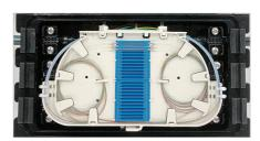
12. Separate the fibers to splice and arrang the rest. Measure the fiber length and cut the fibers to splice. Splice the fibers in order and place the spliced fibers in the splice holder. Arrange the fibers on the tray.
